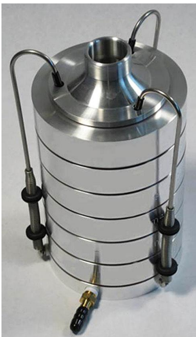
Figure 3: Tisch Six-Stage Viable Sampler
